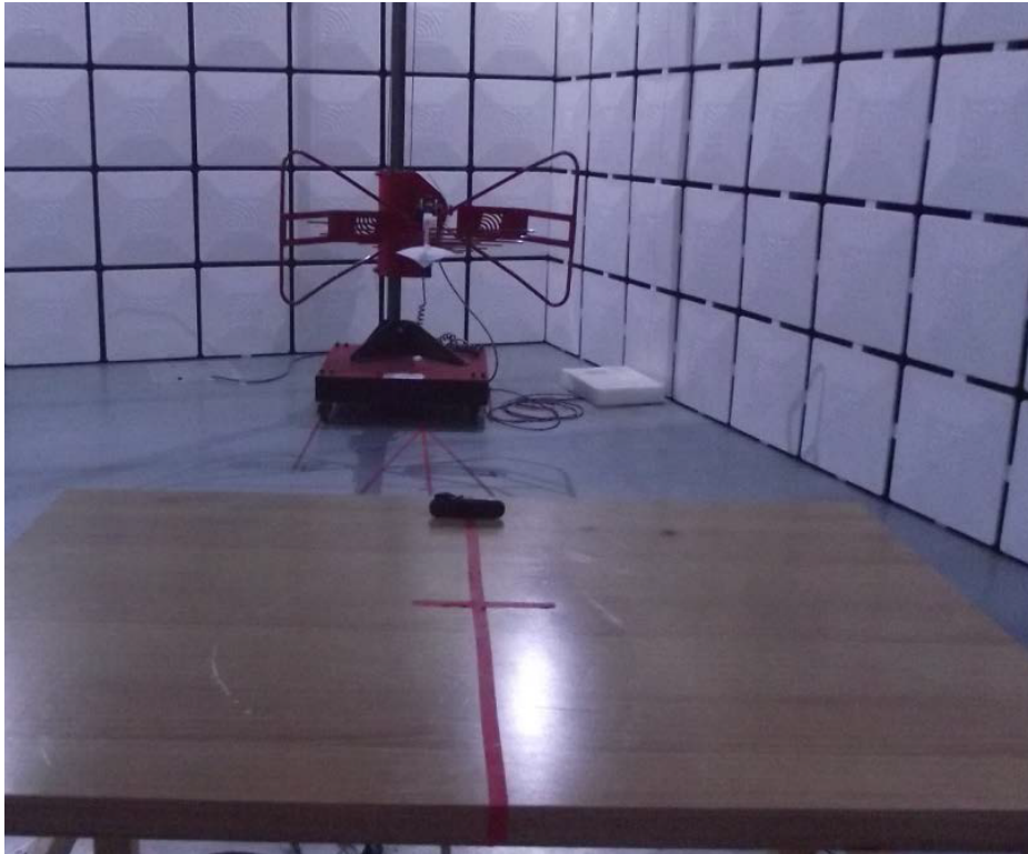
Photo 1 Radiated Emission Test Setup
