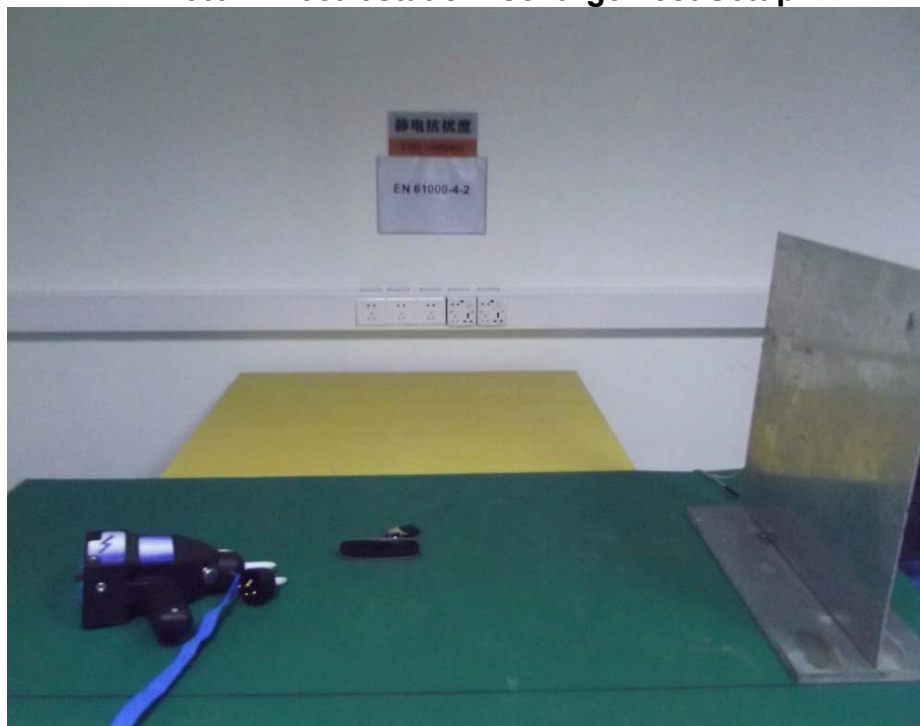
Photo 2 Electrostatic Discharge Test Setup
